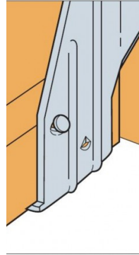
Strong-Grip helps secure the I-joist where no uplift is required.
